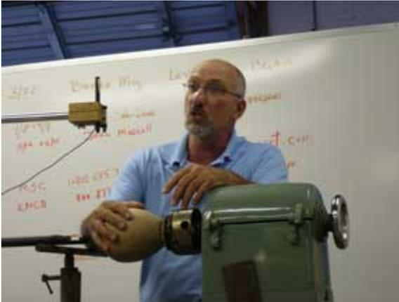
Joe Montagnino enlightened us all with a demonstration on boring bar systems for hollowing. He started by talking about how to mount a blank by determining whether you want to use side or end grain. He then discussed different methods of chucking, including: glue, jam chucks and face plates, etc. Joe said face plates can cut the grain of the wood and dislodge the screws. He also said that some chucks use a 45 degree angle and some use a dove tail. Glue blocks work best for segmented work.
